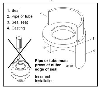
Figure 19. Seal Installation
