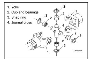
Figure 22. U-Joint Exploded View
