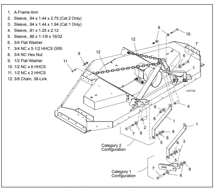
Figure 34. Quick Hitch Kit Installation (Optional)
