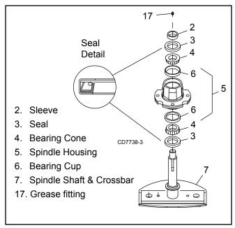
Figure 17. Spindle and Shaft Assembly
