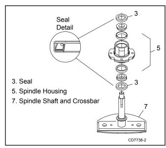
Figure 16. Spindle Disassembly
