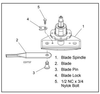
Figure 12. Blade Removal
