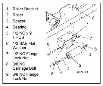
Figure 33. Front Roller Installation
