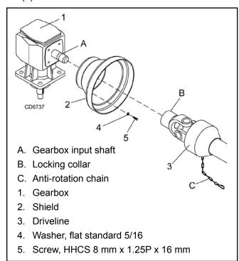
Figure 31. Driveshaft Installation
