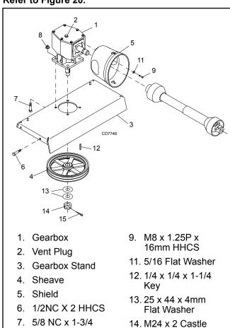
Figure 20. Gearbox Stand Assembly
