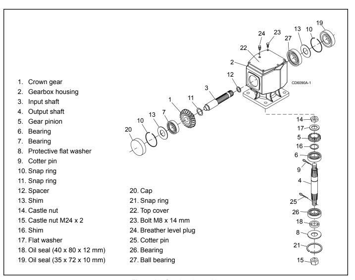
Figure 18. Gearbox Assembly
