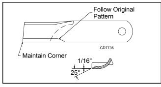
Figure 14. Blade Sharpening
