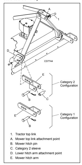
Figure 7. Top Link Adjustment
