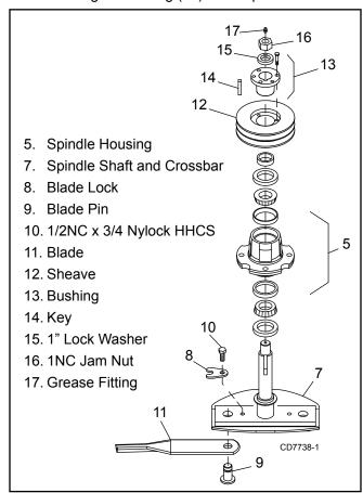
Figure 15. Sheave and Blade Assembly
