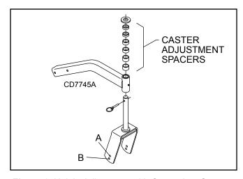
Figure 6. Height Adjustment with Caster Arm Spacers
