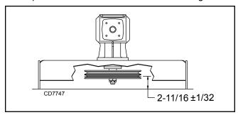
Figure 21. Drive Sheave Installation
