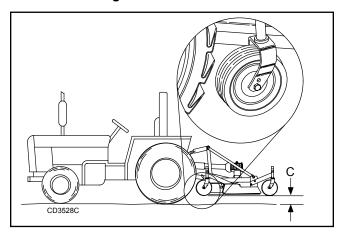
Figure 8. Front Caster Wheel Interference Check
