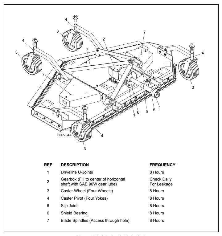
Figure 10. Lubrication Points & Chart
