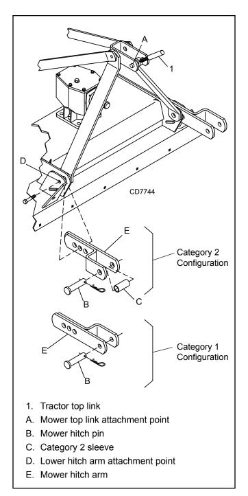
Figure 30. Hitch Arm Installation
