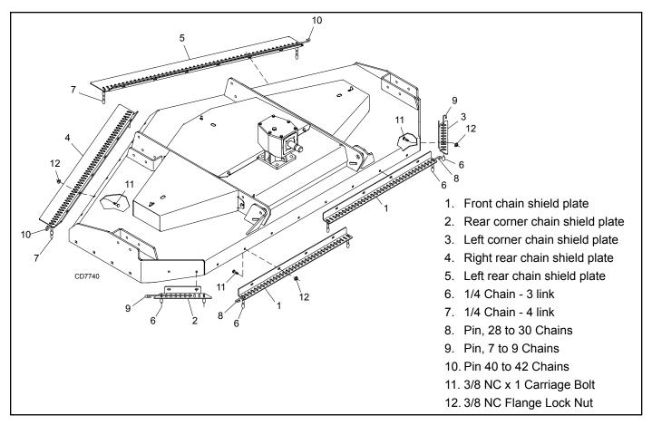
Figure 32. Chain Shield Installation
