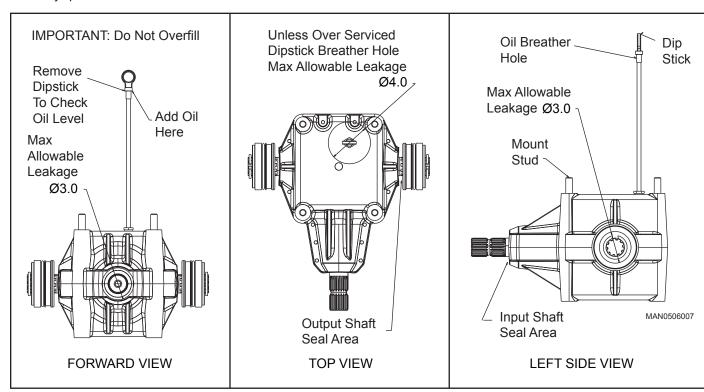
Figure 30. Acceptable Oil Leakage
