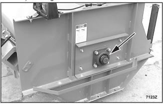
Figure 25. Rotor End Bearing Lubrication Point
