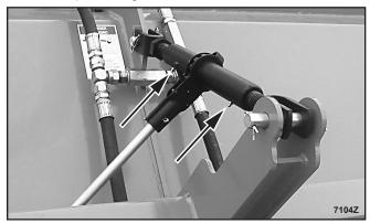
Figure 29. Ratchet Lubrication Points
