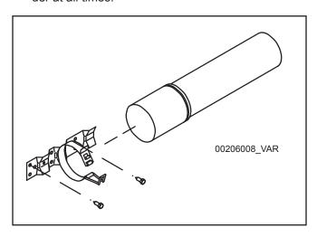
Figure 47. Clamp-Style Manual Tube Assembly
