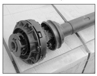
Figure 39. Weasler Modular Friction Clutch (24K)
