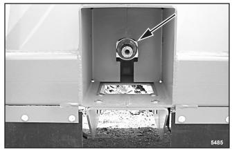
Figure 43. Gearbox Input Shaft
