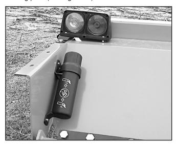
Figure 46. One-Piece Style Manual Tube Installed
