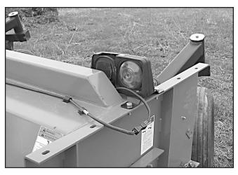
Figure 51. Safety Light Installed - Front View
