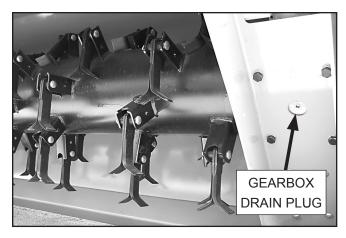
Figure 31. Drain Plug (Underside of Unit)
