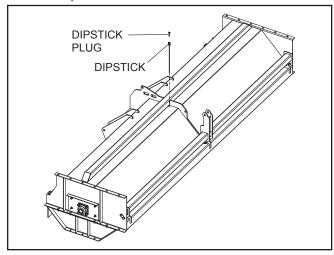
Figure 40. Dipstick Shipping Plug Removal
