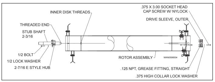
Figure 38. Stub Shaft Assembly
