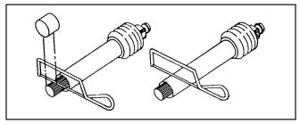
Figure 5. Cutting the Driveline Shaft
