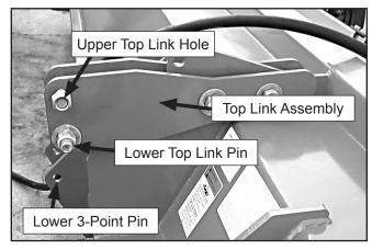
Figure 3. 3-Point Hitch Attachment
