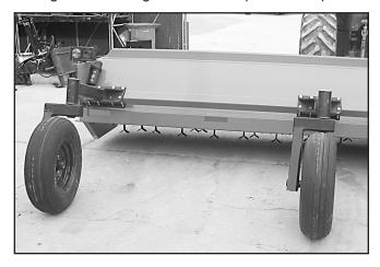
Figure 41. Wheel Assembly Installed
