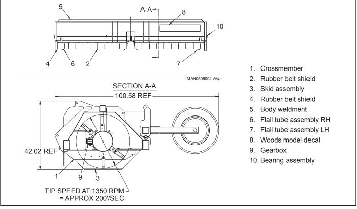
Figure 1. Flail Shredder Principal Components
