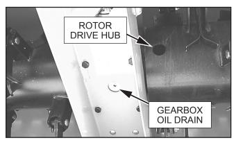
Figure 27. Gearbox Oil Drain Location
