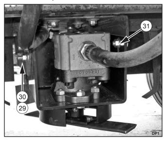
Figure 54. Motor Assembly Installed
