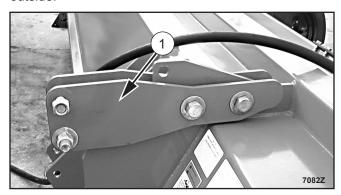
Figure 42. Floating Upper Mast Installed
