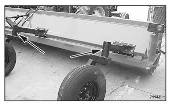
Figure 26. Wheel Rockshaft Bearing **Lubrication Points**
