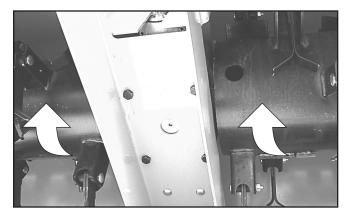
Figure 37. Rotor Direction of Rotation
