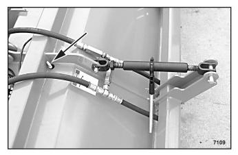
Figure 24. Gearbox Oil Fill Location
