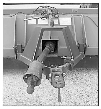
Figure 7. Attaching to Pull-Type Model
