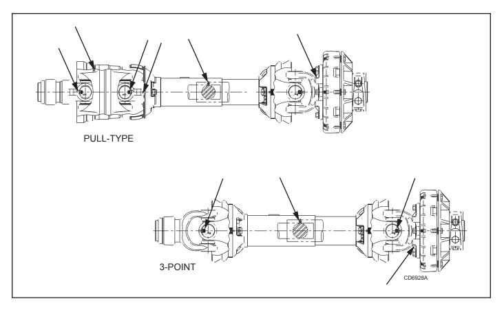
Figure 22. PTO Driveline Lubrication Points
