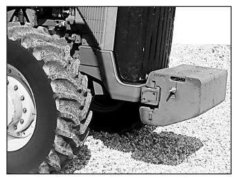
Figure 2. Tractor Front Weight
