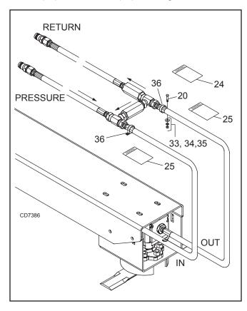
Figure 57. Hose Clamp Installation
