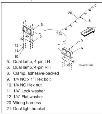
Figure 49. Safety Light Kit Diagram (Non-End Tow)
