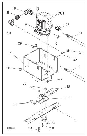
Figure 53. Motor Assembly
