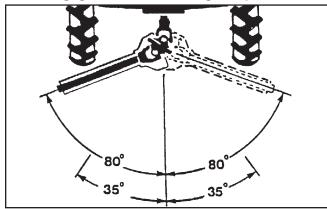
Figure 19. CV Joint Angles
