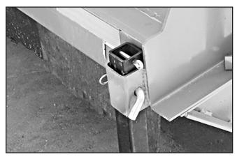
Figure 44. Front Stands Installed
