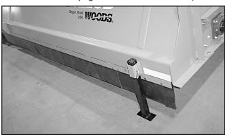
Figure 35. Front Rubber Shield Flaps
