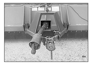
Figure 45. Pull-Type Hitch Installed
