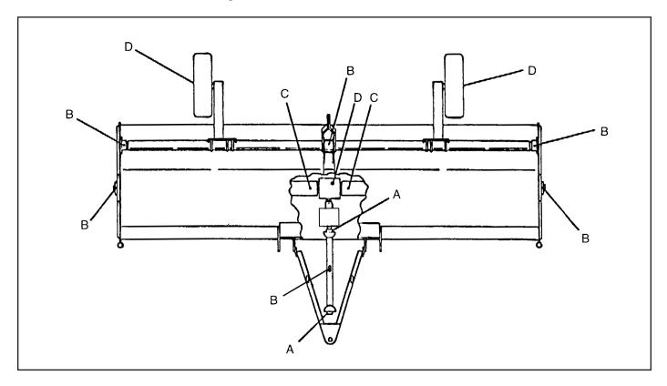
Figure 23. Lubrication Points
