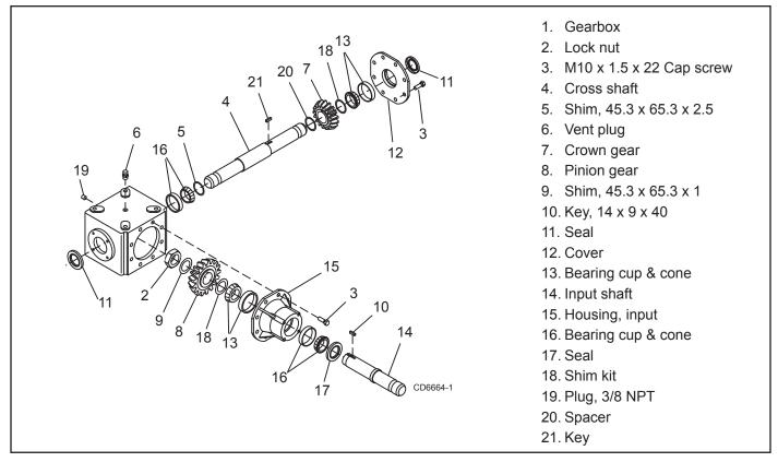
Figure 21. Center Gearbox Assembly
