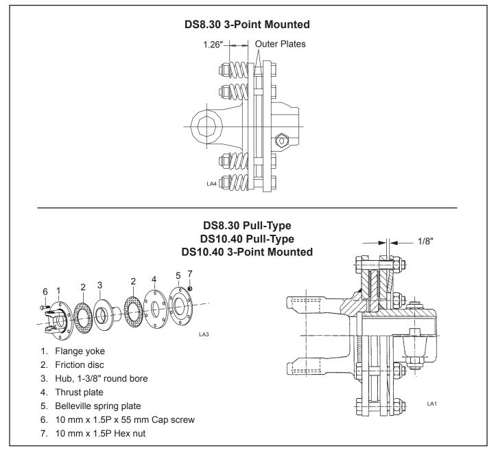
Figure 14. Slip Clutch Assembly
