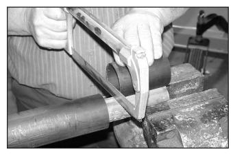
Figure 8. Cut Shaft to Length
