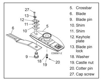
Figure 23. Blade Removal
