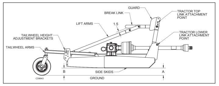
Figure 9. Cutting Height Adjustment
