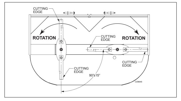
Figure 26. Crossbar Timing - Bottom View
