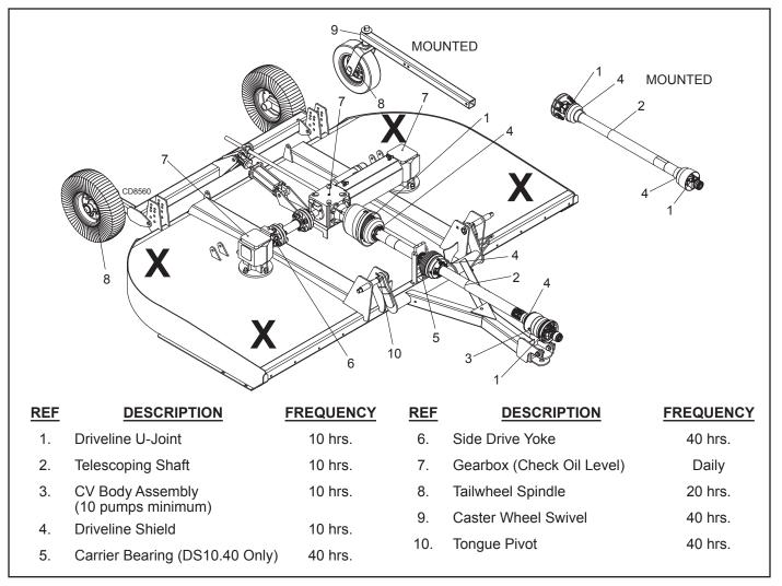
Figure 11. Jackstand Placement and Lubrication Points
