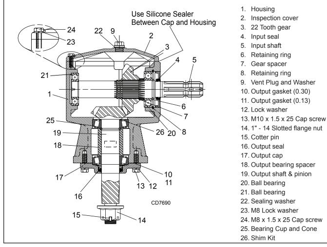
Figure 19. DS8.30 Gearbox Assembly
