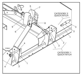
Figure 2. DS8.30 Standard and Quick Hitch Connection
