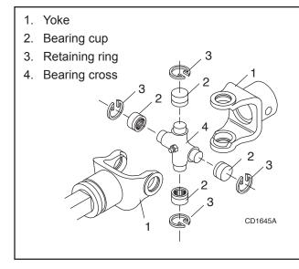
Figure 27. Universal Joint Parts Breakdown
