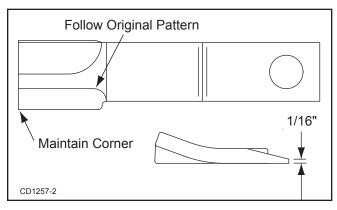
Figure 13. Sharpen Blade Cutting Edge
