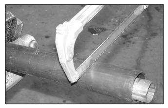
Figure 7. Cut Shield
