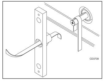
Figure 25. Example of Crossbar and Gearbox Shaft
