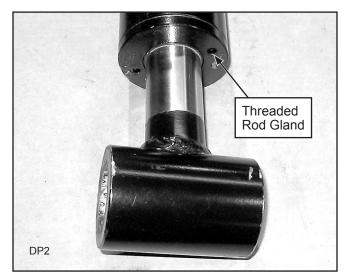
Figure 14. Threaded Rod Gland Cylinder
