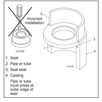
Figure 11. Seal Installation
