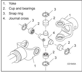
Figure 20. U-Joint Exploded View
