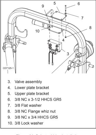
Figure 31. Selector Valve Installation
