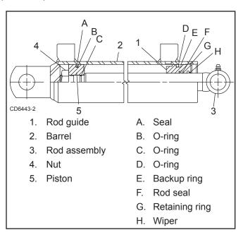
Figure 19. Swing Cylinder Components
