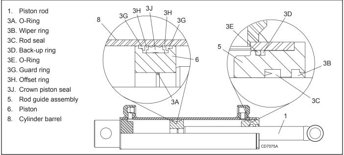
Figure 18. 1021509 Hydraulic Cylinder
