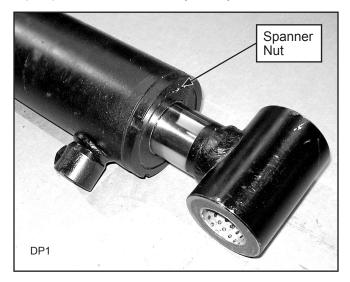
Figure 13. Spanner Nut Cylinder
