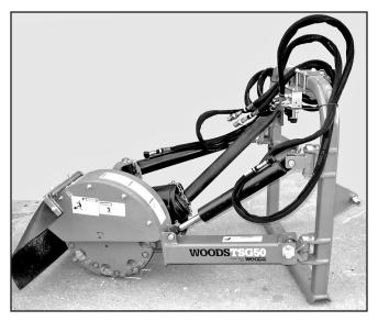
Figure 4. Stump Grinder in Storage Position
