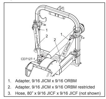
Figure 28. Hose and Fitting Installation
