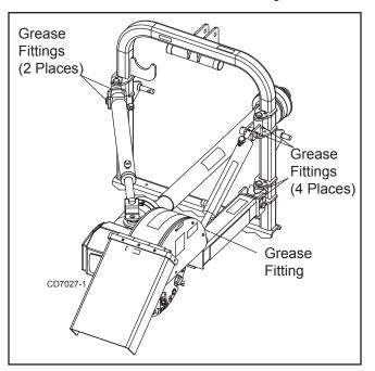
Figure 5. Lubrication Points
