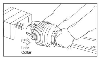
Figure 2. Lock Collar Connection
