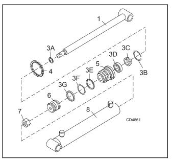
Figure 15. Spanner Nut Cylinder Assembly
