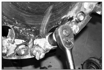
Figure 6. Tooth Installed
