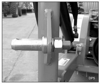
Figure 27. Cat 2 Hitch Pin Installed -Right Side Shown
