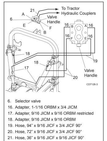
Figure 30. Hydraulic Hose and Fitting Installation
