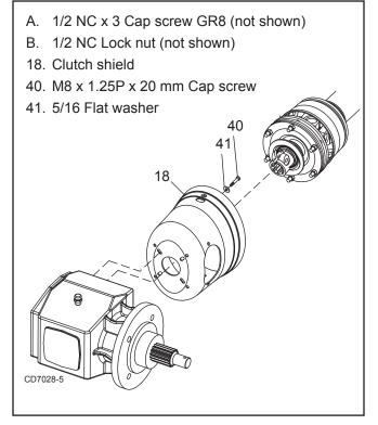
Figure 26. Slip Clutch Driveline Installation
