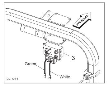
Figure 33. Harness to Valve Assembly Connection
