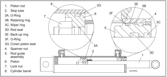
Figure 16. Spanner Nut Cylinder Assembly
