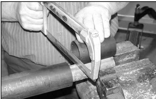
**Figure 6.** Cut Shaft to Length
