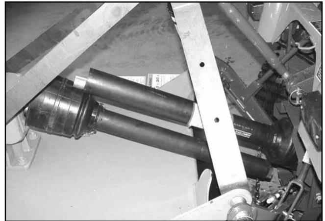
**Figure 3.** Drive Halves Placed Parallel
