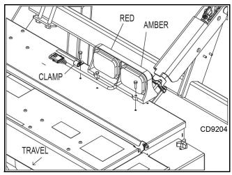
Figure 31. LED Red and Amber Lamp Installation
