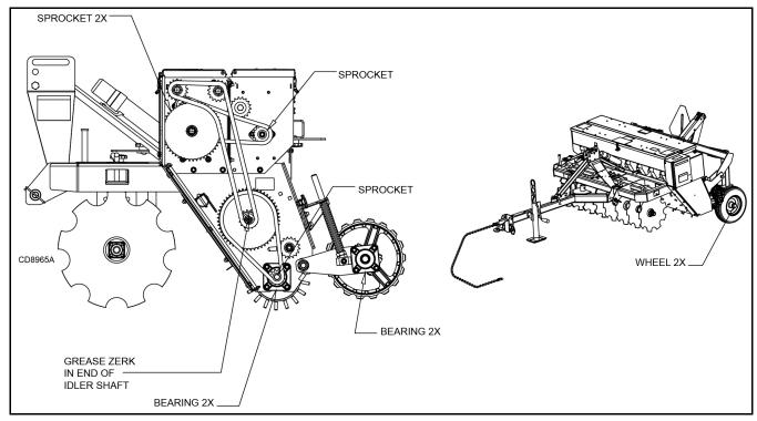
Figure 29. Lubrication Points
