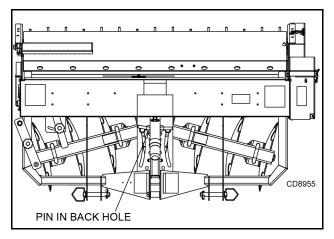
Figure 10. Disc in Angled Position (60" Seeder Shown)
