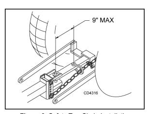
Figure 3. Safety Tow Chain Installation
