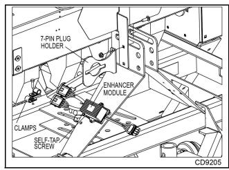
Figure 32. Intermediate Harnesses Connection
