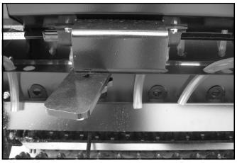
Figure 20. Legume Seed Rate Adjustment Lever
