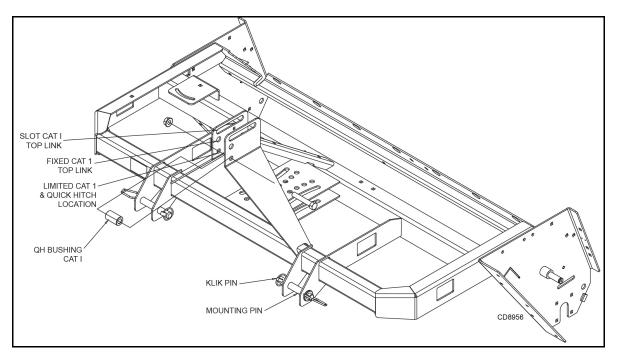
Figure 2. Seeder Hitch Positions
