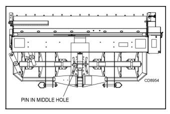
Figure 9. Disc in Straight Position (60" Seeder Shown)
