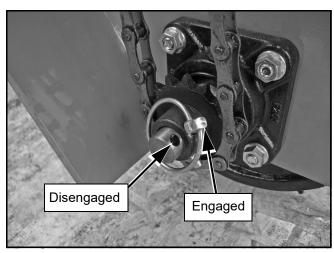
Figure 12. Main Chain Drive Disconnect
