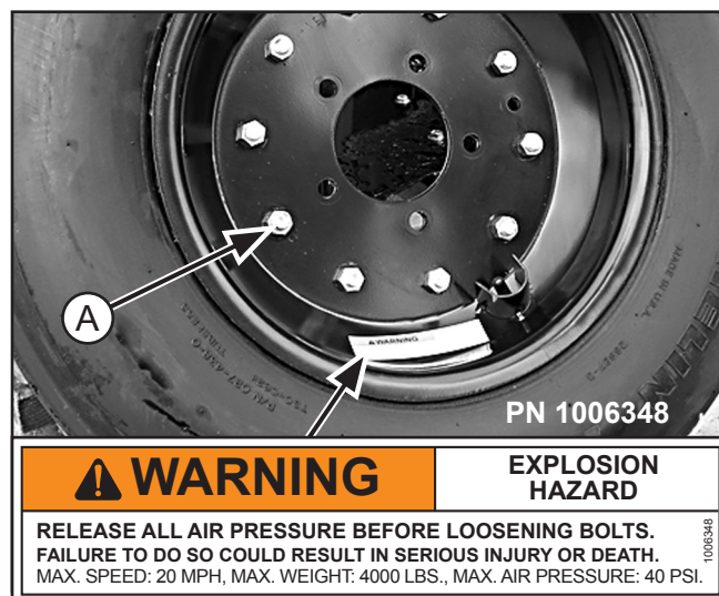
Figure 21. Split Rim Tire Servicing
