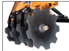
2. Or, choose adjustable disc blades that cut into and work the soil. Easily adjust the blade angles to till more aggressively depending upon soil conditions.
