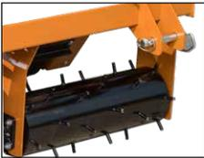
1. Choose a spiked roller with adjustable angles that will penetrate thatch and aerate lawns, or angle it to break up the surface and remove stands of turf.
