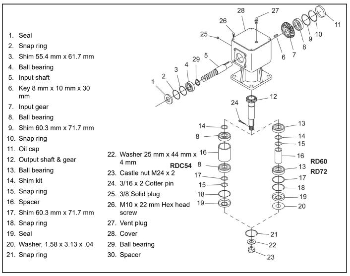
Figure 16. Gearbox Assembly
