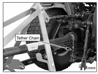
Figure 3Attach Mower to Tractor
