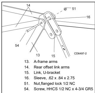
Figure 26. Top Link Assembled
