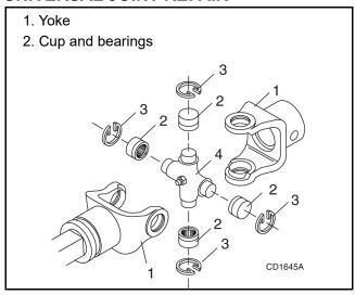
Figure 18. U-Joint Exploded View
