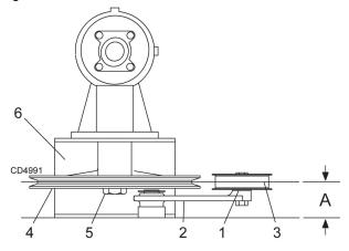
Figure 17 Drive Sheave Installation
