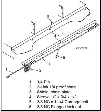
Figure 28. Chain Shield Installed (RDC54 Only)
