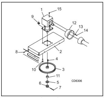
Figure 15. Gearbox Stand Assembly
