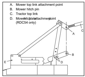
Figure 4. Top Link Adjustment
