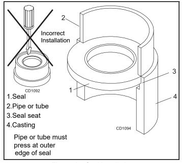
Figure 14. Seal Installation
