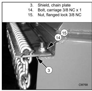
Figure 27. Chain Shielding Installed (RD60 & RD72 Only)
