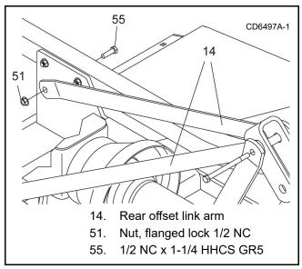
Figure 25. Right Rear Offset Link Installed
