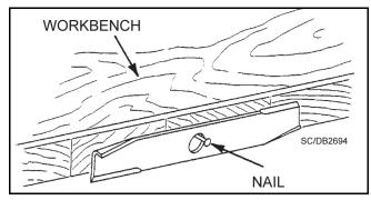
Figure 10. Blade Balancing
