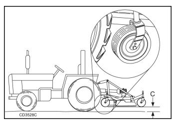
Figure 5. Front Caster Wheel Interference Check
