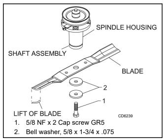
Figure 11. Blade and Spindle Assembly
