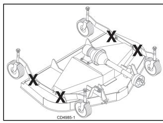
Figure 12. Jackstand Placement
