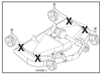
Figure 7. Jackstand Placement
