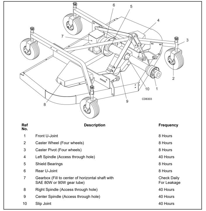
Figure 8Lubrication Points & Chart
