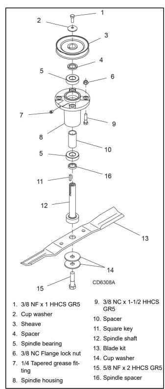
Figure 13. Blade Spindle Assembly
